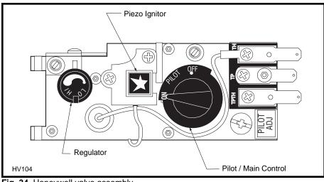
Fig. 34 Honeywell valve assembly.
